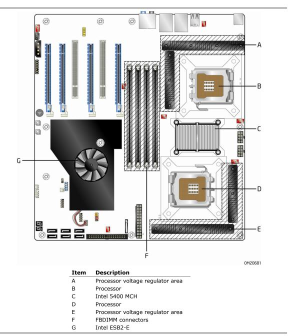
Figure 17. Localized High Temperature Zones
